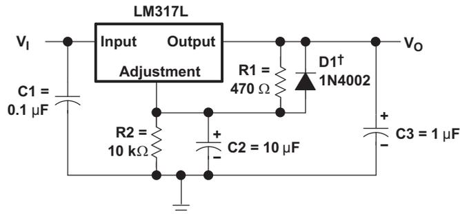
Figure 3. Regulator Circuit With Improved Ripple Rejection
