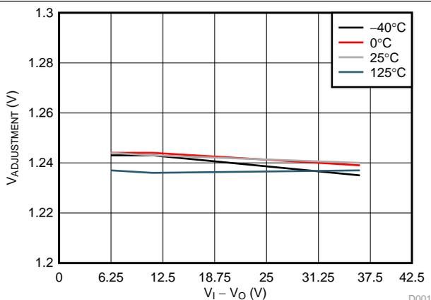
Figure 2. Adjustment Voltage Relative to Output Over Temperature
