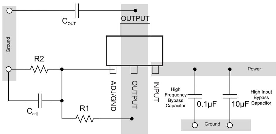
Figure 11. Layout Diagram
